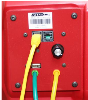
Figure 17: color-coded tubing connections (green and yellow) and Control Cable
