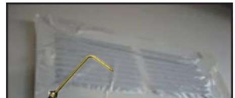
Figure 15: A Static Pressure Probe attached to a pressure tube allows the measurement of pressure without disturbances due to turbulence.
