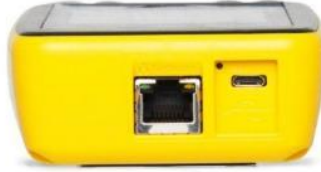
Figure 16: Electrical connections on the bottom of the gauge include Network (Ethernet) Cable that goes from the DM32 to a PC (if Retrotec PC software is used for data collection), micro USB cable for PC software and/or charging, and a reset button.
