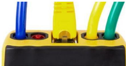
Figure 14: Pressure ports on the top of the gauge are color-coded to match the tubing
