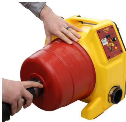
Figure 12: Install Flex Duct over the fan inlet, covering the Range Rings, for depressurization. Later systems have a 2.5 inch connector instead of the 4 inch (100 mm) shown.
