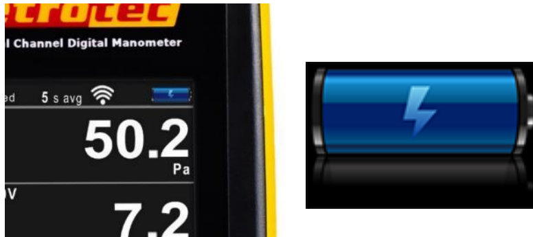
Figure 10: The screen of the DM32 while the batteries are being charged.
