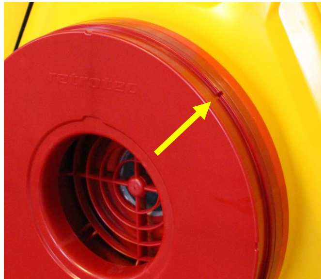
Figure 4: Self-referencing pressure pickup connect to the green port and must never be taped over.
