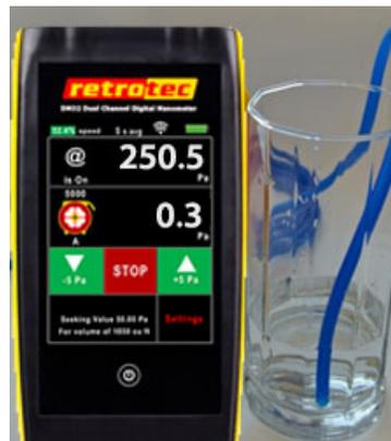
Figure 70: Gauge displaying 250.5 Pa (or 1 in WC).
