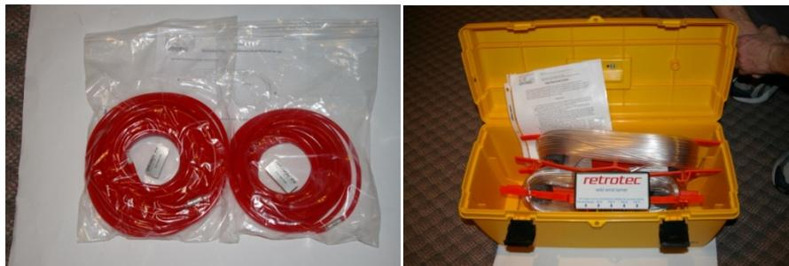
**Figure 69: Wind damping kits; basic (left) and deluxe (right).**
