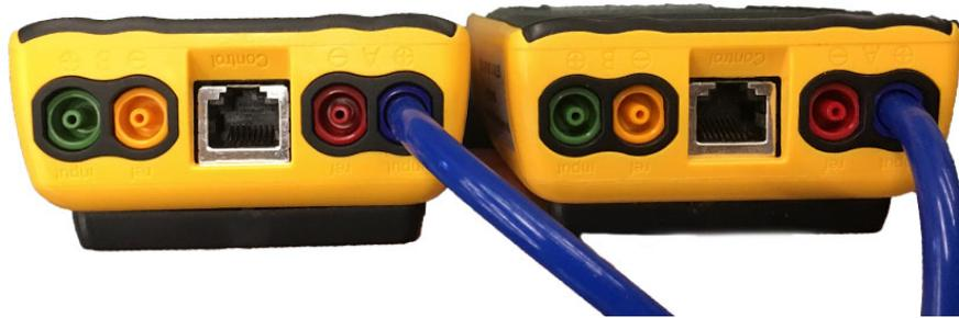
**Figure 66: Gauge field check configuration: Cross gauge check**
