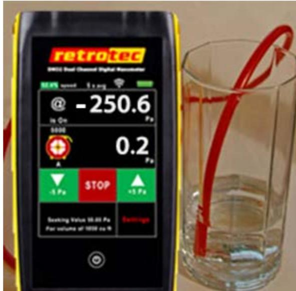
Figure 71: The gauge displaying a negative pressure (-250.6 Pa).
