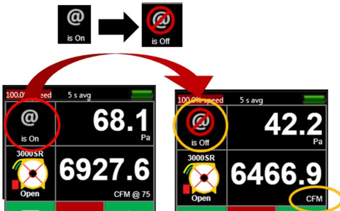
Figure 32: Turn [**@ Pressure**] off, leaves fan running
