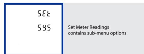
To enter set-up menu, hold the **E** button for 3 seconds, until the screen appears.
