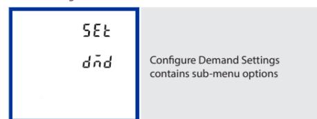
To enter set-up menu, hold the **E** button for 3 seconds, until the screen appears.
