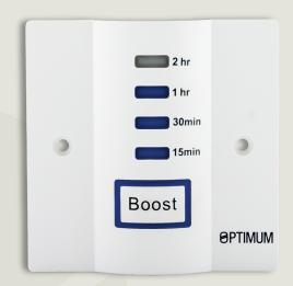
OP-EBT2 IS A ONE-BUTTON BOOST TIMER. THERE ARE FOUR PRE-SET TIMED OUTPUTS. SUITABLE FOR INSTALLATION ON A SURFACE OR IN-WALL PATTRESS BOX. THE ELECTRONIC TIMER CONTROLS AN INTERNALLY LINKED OUTPUT RELAY, WITH A RESISTIVE RATING OF 16 AMPS. AN EARTH PARK TERMINAL IS PROVIDED. SURFACE-RUN CORD OUTLET WITH CABLE RESTRAINT. PRESS UP TO 4x TO SELECT BOOST OUTPUT, PRESS AGAIN TO CANCEL.
