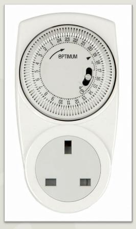
OP-TIP1000 IS A CAPTIVE-TAPPET 24-HOUR PLUG-IN TIME SWITCH. EACH TAPPET OPERATES FOR 15 MINUTES. THE TIMER IS SUITABLE FOR USE IN BS1363 SOCKETS. THE 24 HOUR DIAL CONTROLS THE OUTPUT TO A BS1363 COMPLIANT SHUTTERED SOCKET, AND HAS A RESISTIVE RATING OF 13 AMPERES.
