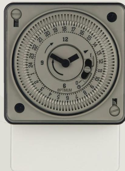
OP-TS211.1 IS A CAPTIVE-TAPPET 24-HOUR TIME SWITCH. EACH TAPPET OPERATES FOR 15 MINUTES. THE TIMER IS SUITABLE FOR SURFACE, PANEL AND DIN-RAIL MOUNTING. THE 24 HOUR DIAL CONTROLS A VOLT-FREE CHANGEOVER SWITCH, WITH A RESISTIVE RATING OF 16 AMPERES. THERE IS AN INBUILT RE-CHARGEABLE CELL TO KEEP THE TIMER RUNNING IN THE EVENT OF A LOSS OF MAINS POWER.
