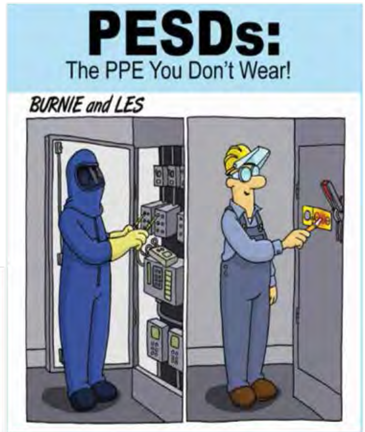
Adding PESD'S reduces the risk of Arc Flash
